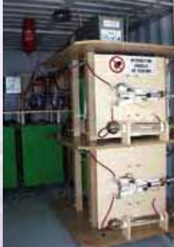
Lightning wave generator 10 / 350
